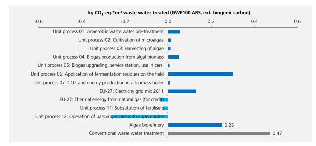
Figure 4-1: Global warming potential per m<sup>3</sup> of waste water treated (GWP100 AR5 excl. biogenic carbon)
