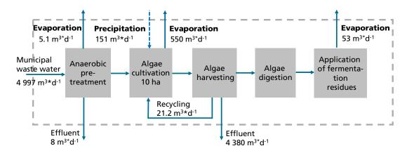
Figure 3-4: Blue water balance of the algae biorefinery; values refer to one day of operation, dotted arrow indicates green water which is not considered
