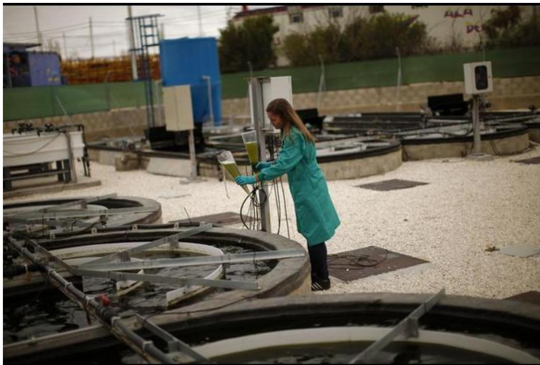
Aqualia's All-gas project researcher Laureano collects water samples with Imhoff cones from a tank at a waste-water treatment plant in Chiclana de la Frontera
